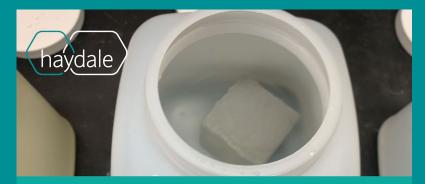
The Quartz sealed material is not bubbling with no degradation taking place.
